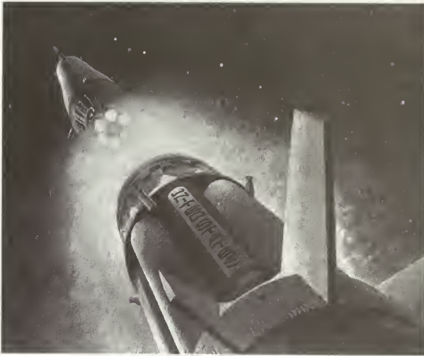
Top left, Saturn I SA-4 rises from the launch pad on 28 March 1963. The last of the Block I vehicles, it has no aerodynamic fins as does SA-5, which sits on the pad at top, right. At left is an artist's conception of S-IV stage separation in space, with the six RL-10 engines kicking the payload into orbit.
